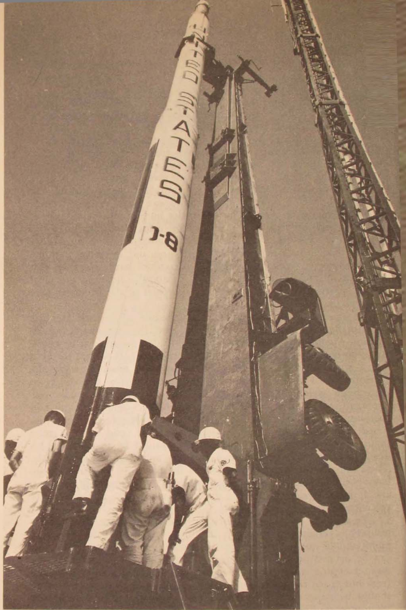
A "blue suit" launch capability has been developed in support of the Air Force Blue Scout booster program. Versatility of the Blue Scout family, derived from the NASA Scout program, permits use of solid-propellant rockets in a variety of projects for which higher performance and more expensive rockets are not needed.
