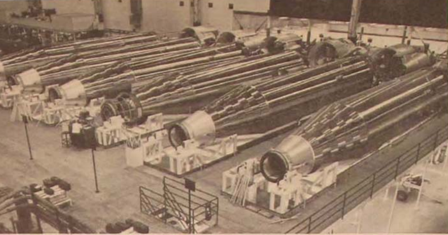
Atlas intercontinental ballistic missiles on the production line or "dock" at the General Dynamics/Astronautics plant, San Diego. These thin-skinned cylinders must be kept under pressure constantly until they have been fueled.
